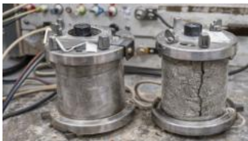
Figure 17 RCPT test Table 4 RCPT test results
