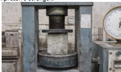
Figure 8 Compressive strength test
